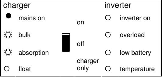
The AC voltage on AC-in-1 or AC-in-2 is switched through, and the charger operates in equalisation mode.
