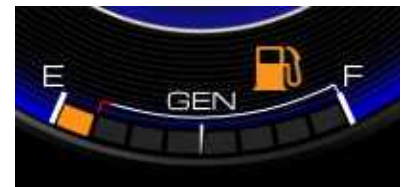
Fuel level low – generator will run out of fuel
